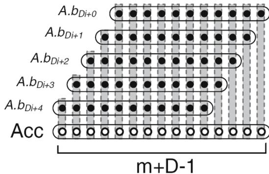
Figure 2. Multiple digit adder core [3]
