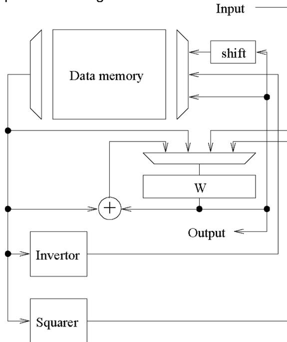
Figure 3. Main architecture data path
